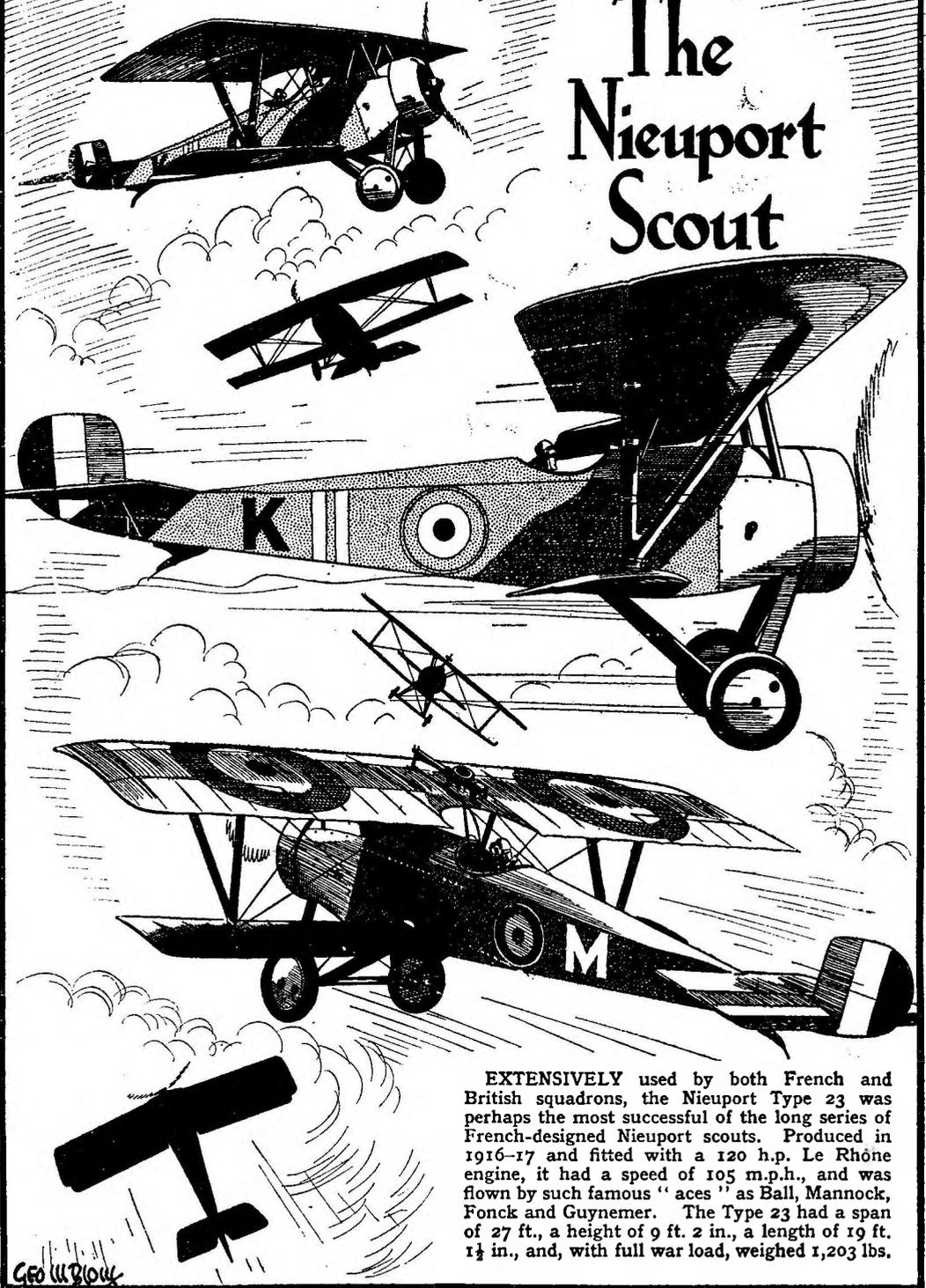
EXTENSIVELY used by both French and British squadrons, the Nieuport Type 23 was perhaps the most successful of the long series of French-designed Nieuport scouts. Produced in 1916-17 and fitted with a 120 h.p. Le Rhône engine, it had a speed of 105 m.p.h., and was flown by such famous "aces" as Ball, Mannoek, Fonck and Guynemer. The Type 23 had a span of 27 ft., a height of 9 ft. 2 in., a length of 19 ft. 1½ in., and, with full war load, weighed 1,203 lbs.
